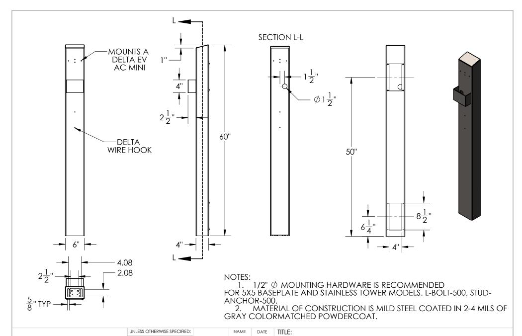
DIMENSIONS ARE IN INCHES TOLERANCES: FRACTIONAL ± 1/32 DRAWN INSTALLATION CHECKED ANGULAR: ±2° TWO PLACE DECIMAL ±0.010
