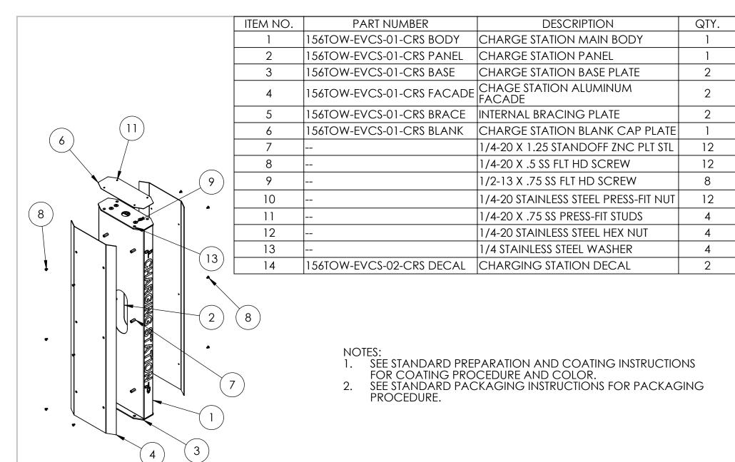
DIMENSIONS ARE IN INCHES DRAWN **ASSEMBLY** TOLERANCES: CHECKED FRACTIONAL±1/32 ANGULAR: ±2° TWO PLACE DECIMAL ±0.010 SIZE PART NO. **REV** THREE PLACE DECIMAL ±0.005 156TOW-EVCS-01-CRS INTERPRET GEOMETRIC TOLERANCING PER: WFIGHT: 75.581 NO SCALE SHEET 2 OF 10 ASME Y14.5 -2009
