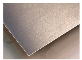
Despite its name, stainless steel can and does stain, so it needs to be cleaned to prevent surface rusting or "pitting" and to preserve its natural corrosion resistance. Stainless steel actually thrives with frequent cleaning, and, unlike some other materials, it is impossible to "wear out" stainless steel by excessive cleaning.
